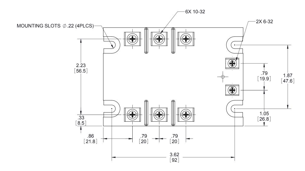
Tolerances: ± 0.02 in / 0.5 mm. All dimensions are in: inches [millimeters]
